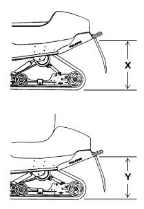
To determine sag, commonly referred to as ride-in, subtract measurement Y from X (sag=X-Y). Adjust sag by rotating the torsion spring preload cams located on the rear torque arm. Use the illustration for reference. The ideal amount of Sag for the EDGE rear suspension is four inches (X-Y=4).
